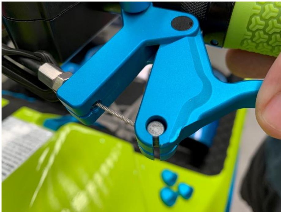
★ [IMG6060: THROTTLE WHEEL GREASE POINT]
