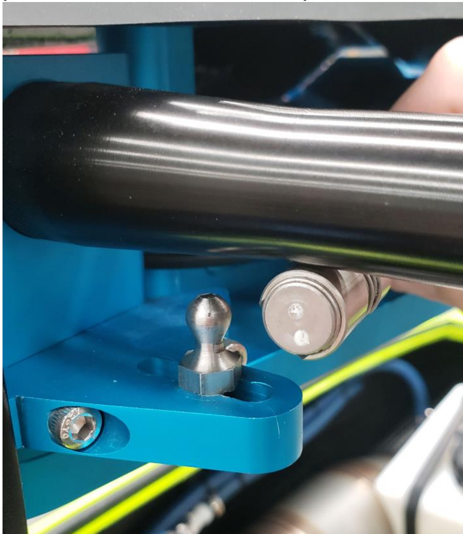
★ [IMG6070: STEERING BALL JOINT GREASE LOCATION]
