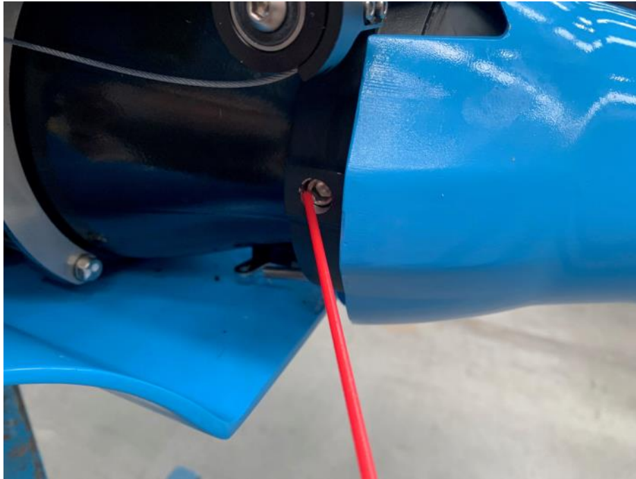
★ [IMG6040: HOOD LATCH SPRAY POINTS]
